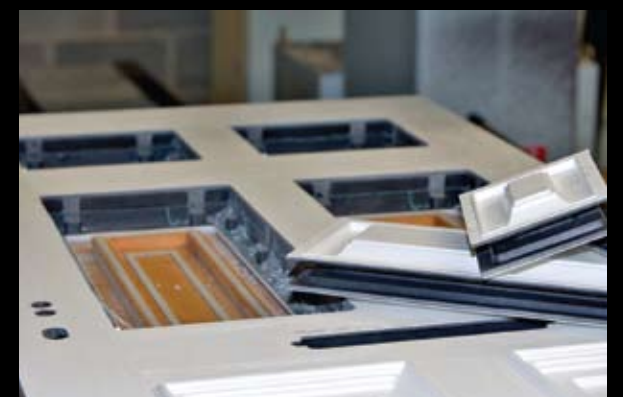
Door after routing operation
