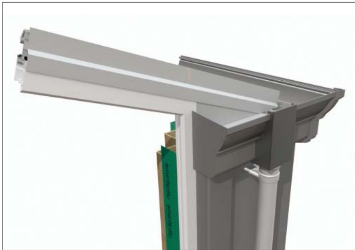
SHORT RETURN WITH CORNICE. If unable to return back to house wall use Elephants Trunk outlet positioned centrally on column.
