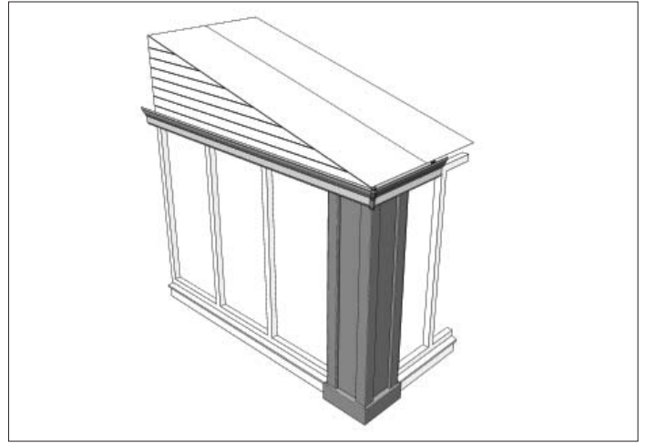
Self manufactured firring* - see illustration B on p31
