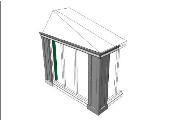
Hipped end with abutment
