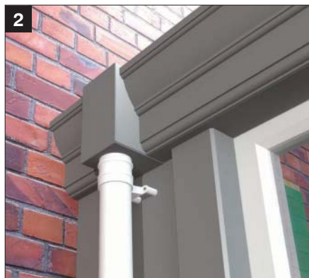
2 Elephants trunk outlet. If it is not possible to have full height columns.
