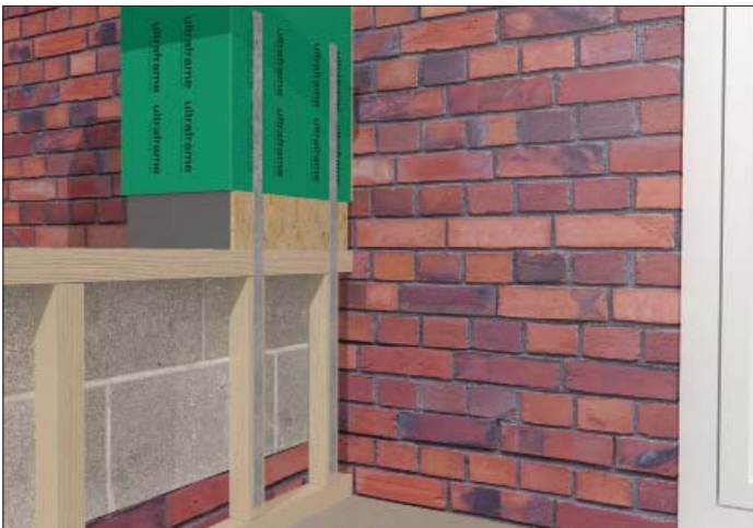
STRAPS MUST LINE UP WITH STUDWORK
