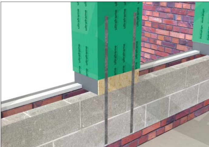
INLINE Fasten straps down inside of wall of inline column. Use suitable fixing.
